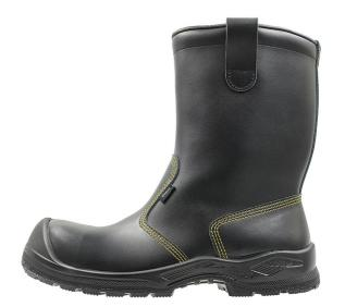
Mid-calf boots made of durable and water-repellent PU coated leather. Pull tabs on the back make the boots easy to put on. The foot is protected by a composite toecap and perforation-resistant steel midsole. Flexible polyurethane soles provide excellent traction and withstand oil and many chemicals. ESD approved.
