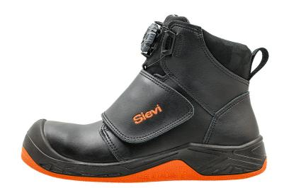
The heat-resistant nitrile rubber sole can withstand temperatures up to 300°C. The smooth special sole does not leave marks or collect dirt, making the shoe ideal for pitch and asphalt work. The lightweight aluminium toe cap and steel midsole provide protection even in harsh conditions. The BOA® Fit System makes effortless to put on and take off. Heat-resistant stitching. Antistatic and ESD approved.
