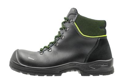
Lace-up ankle boots made of durable PU-coated leather with composite toecaps and penetration resistant steel midsoles. Polyurethane soles are resistant to oil and a number chemicals and absorb shocks effectively. Breathable and structured insoles and 3D-dry® lining improve ventilation and make the boots comfortable to wear. ESD-approved.
