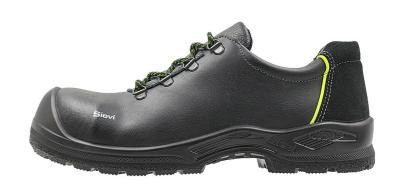
Lace-up shoes made of durable PU-coated leather with composite toecaps and perforation-resistant steel midsoles. Polyurethane soles are resistant to oil and a number chemicals and absorb shocks effectively. Breathable and structured insoles and 3D-dry® lining improve ventilation and make the shoes comfortable to wear. ESD-approved.
