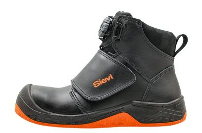
The heat-resistant nitrile rubber sole can withstand temperatures up to 300°C. The smooth special sole does not leave marks or collect dirt, making the shoe ideal for pitch and asphalt work. The lightweight aluminium toe cap and steel midsole provide protection even in harsh conditions. The BOA® Fit System makes effortless to put on and take off. Heat-resistant stitching. Antistatic and ESD approved.
