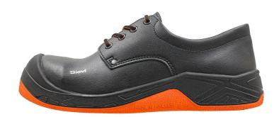
The nitrile rubber sole can withstand temperatures up to 300°C. The smooth special sole does not leave marks or collect dirt, making the shoe ideal for pitch and asphalt work. The lightweight aluminium toe cap and steel nail guard provide protection even in harsh conditions. The wear-resistant polyamide surface of the Green Comfort insole wicks moisture from the foot surface to the lower layer of the insole. Heat-resistant stitching.
