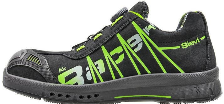
An S3 protection class shoe with SieviAir® sole, BOA® Fit System, penetration-resistant steel midsole and aluminium toe cap. The FlexEnergy® component, the world's most advanced shock-absorbing heel, stores kinetic energy and gives a greater than 55% energy return. The SieviAir® sole dissipates the perspiration created by the heat of the feet through special ducts.
