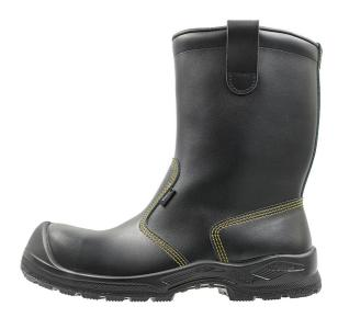
Mid-calf boots made of durable and water-repellent PU coated leather. Pull tabs on the back make the boots easy to put on. The foot is protected by a composite toecap and penetration resistant steel midsole. Flexible polyurethane soles provide excellent traction and withstand oil and many chemicals. ESD approved.
