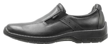
The upper is made from black top-grain leather, which retains its shape and repels water. Elastic on the side makes it easier to put on. The flexible Flexstep® sole is made of polyurethane and absorbs impacts to the back and feet. The removable Sievi Comfort insole is antistatic and ESD compliant, breathable and machine washable at 40 °C. ESD approved.
