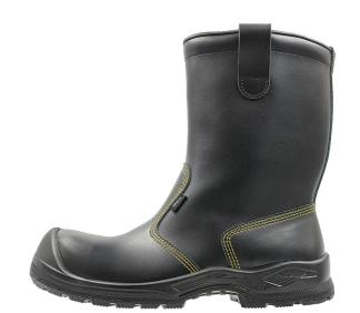
Mid-calf boots made of durable and water-repellent PU coated leather. Pull tabs on the back make the boots easy to put on. The foot is protected by a composite toecap and penetration resistant steel midsole. Flexible polyurethane soles provide excellent traction and withstand oil and many chemicals. ESD approved.
